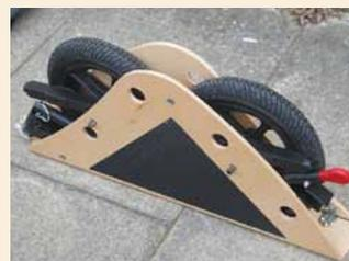
3 Lay the package on its side; its own weight will press onto the axle end buttons, releasing the locking balls and allowing you to fold out the trailer.
