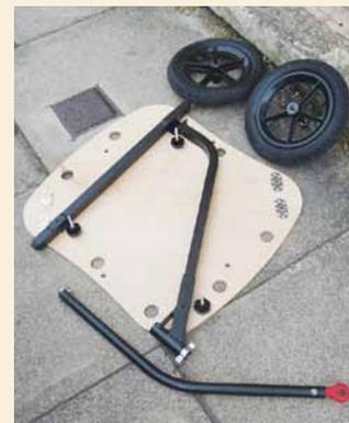
5 The cross and diagonal beams interlock, then there are three thumbscrews to tighten the frame to the trailer bed. Next you just need to slide the drawbar into place. It secures with a quick release and is safety-locked by a spring clip. Finally, just add the wheels and you have a trailer!
