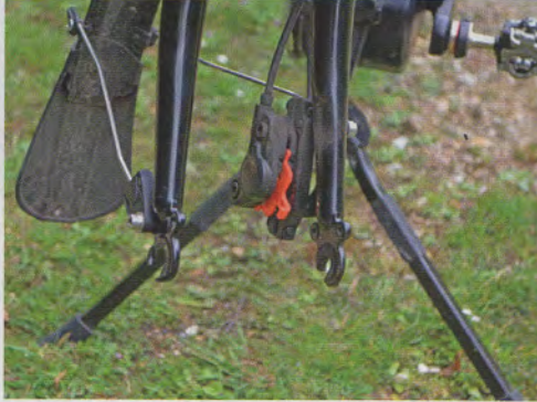
Above: Ease of transport is a key concern for any potential tandem purchase; our test team found it quite manageable to fit the Circe into their BMW 1 Series. Below: A nice feature of the center stand is the ease of removing wheels for packing the bike, or for tire repairs on the road.
