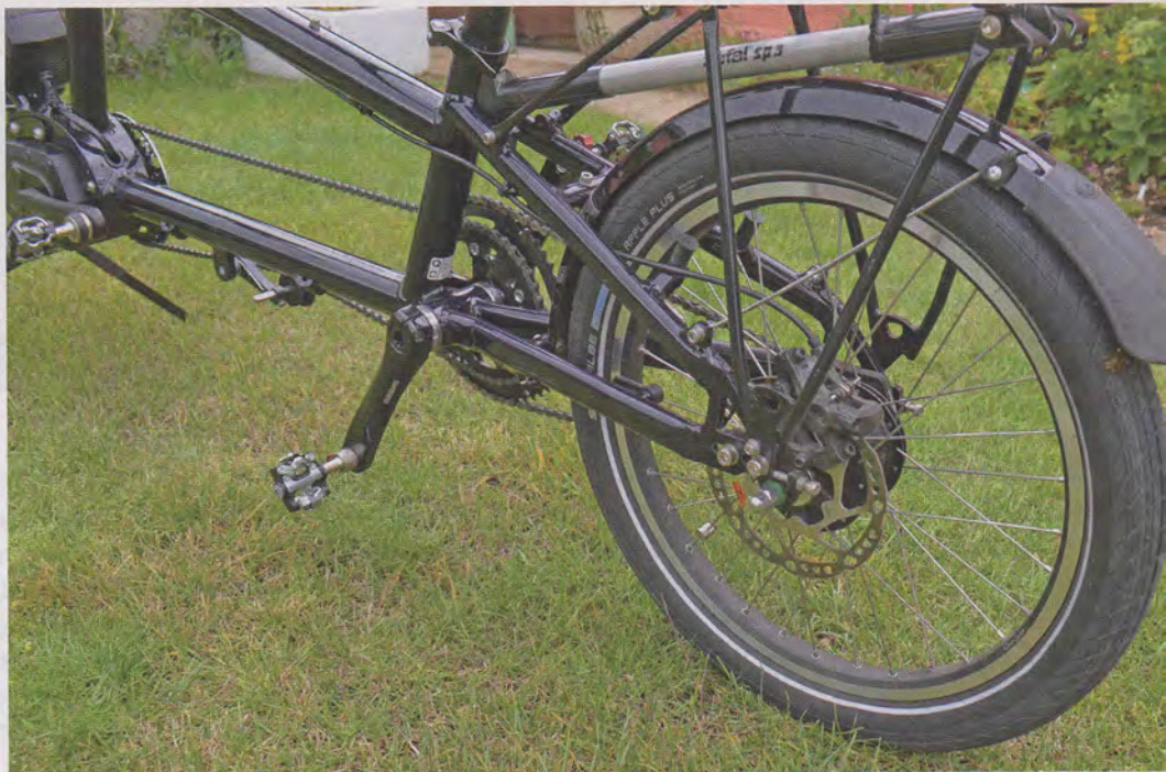
Above and right: Shimano Deore hydraulic disc brakes were found to provide more than adequate power in the hills of Great Britain's Yorkshire dales. Frame pump is cleverly mounted above the rear fender.
