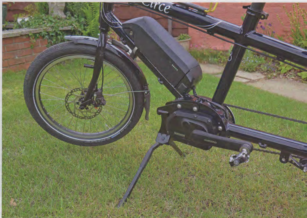
The Shimano STEPS (Shimano Total Electric Power System) motor and battery are the two key elements aboard the Circe tandem. The locking battery pack is removable and can be charged while still on the bike. Green lights visible indicate battery level. Our test team found the center-stand to be a very handy feature.
