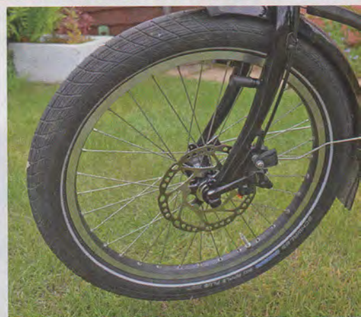
Above and right: Shimano Deore hydraulic disc brakes were found to provide more than adequate power in the hills of Great Britain's Yorkshire dales. Frame pump is cleverly mounted above the rear fender.
