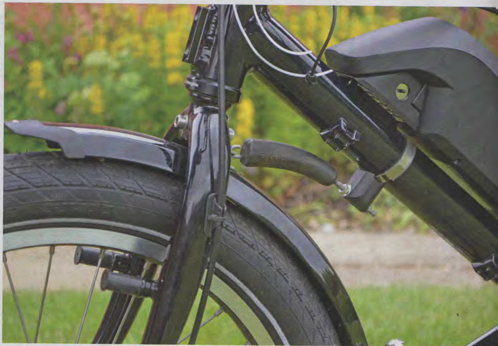
Internal runs for cabling helps clean up the frame; our test team felt removing the extra lugs and mounts for unused equipment would help the bike's aesthetics. Rubber retainer between the frame and fork can be used to keep the front wheel straight when the bike is parked on stand.
