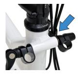
The lower seat mount fits to the frame via a bolt and lever. There are three potential positions for the bolt to be in, depending on the desired position of the seat. The bolt is tightened by rotating the black lever clockwise, whilst holding the nut on the other side. The lever can't rotate fully because of the seat, so it is possible to disengage the lever by pressing the red button and pulling the lever out, allowing it to be rotated freely back to a suitable starting position.
