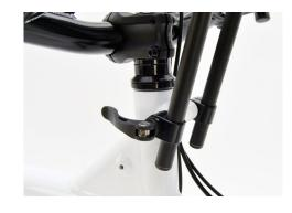
**NOTE** – The P clip holding the cables should be on the inside of the clamps and on the left hand side of the bike.
