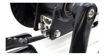
Once the crank assmbly is positioned on the main tube it can be fixed in place using the four M6 hex bolts and a 10mm spanner.
