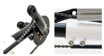
**NOTE** – Tighten the pinch bolts evenly to prevent damage to the frame
