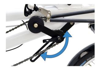
The timing chain can be tensioned by undoing the quick release on the tensioner arm and rotating the arm to take up the slack in the chain. If the tensioner alone can't take up the slack in the chain, it is possible to shorten the timing chain by
