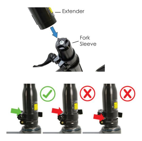
It is possible to orientate the handlebars at 90 deg increments, which can be useful for storing the bike in narrow spaces, or, when transporting the bike by car or train. To do this, the quick release lever needs to be released and the Extender lifted clear of the 4-pointed star, the steerer can then be rotated and reengaged with the 4-pointed star at the desired position.
