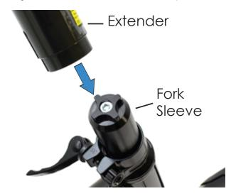
The steerer extender fits to the top of the fork and locates on the 4-pointed star, the slot at the back of the extender should align with the vertical slot on the side of the top cap when the handlebars are pointing forward. Ensure the steerer is fully pushed down before tightening the Q/R.
