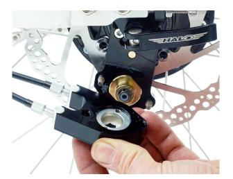
When reinstalling the Rohloff you must orienatate the torque arm such that it aligns with the lower disc brake mounting bolt.
